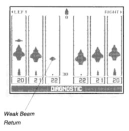
"Diagnostic" is selected with the sonar mode option of the System menu. It is a special screen that displays the raw sonar information being received by each of the six sonar beams. Viewing the information in this manner is helpful when selecting a mounting location for the transducer, or when troubleshooting potential problems.
